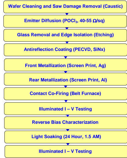
Figure 7: Standard device processing and characterization outline
