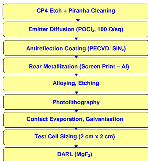
Figure 15: High efficiency device process outline
